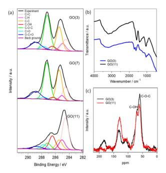
Fig. 1 Characterization of the prepared GO samples. (a) C 1s XPS spectra of GO (3) (GO at pH = 3), GO (7) (GO at pH = 7) and GO (11) (GO at pH = 11), (b) FTIR spectra GO (3) and GO (11), and (c)  $^{13}$ C NMR spectra of GO (3) and GO (11).
