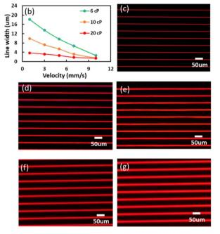
(a) Schematic illustration of the EHD printing system comprising a single nozzle, a movable platform, a conductive platform and a power supply system, (b) and (c-g) fluorescence images of patterned lines with QD ink of 6 cP at printing speeds of 10 mm  $s^{-1}$ , 7 mm  $s^{-1}$ , 5 mm s<sup>-1</sup>, 3 mm s<sup>-1</sup> and 1 mm s<sup>-1</sup>, respectively.
