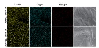
Fig. 6 Representative images of the scanning of carbon, oxygen and nitrogen by SEM-EDS of AcKP<sub>5</sub>NH<sub>2</sub>-CNF (upper panels) and AcKP<sub>10</sub>NH<sub>2</sub>-CNF (lower panels) and the corresponding SEM images (scale bars repre-
