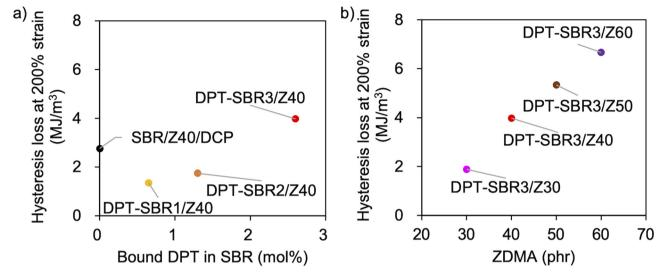
Fig. 13 Hysteresis loss at 200% strain: (a) effect of the amount of bound DPT in the SBR and (b) effect of the amount of loaded ZDMA.
