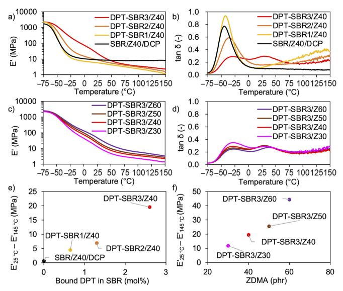
Fig. 9 Temperature dependence of the viscoelasticity: (a) effect of the amount of bound DPT in the SBR on E', (b) effect of the amount of bound DPT in the SBR on tan  $\delta$ , (c) effect of ZDMA content on E', (d) effect of the loaded ZDMA content on tan  $\delta$ , (e) effect of the amount of bound DPT in the SBR on the difference between E' at 25 °C and E' at 145 °C and (f) effect of ZDMA content on the difference between E' at 25 °C and E' at 145 °C.
