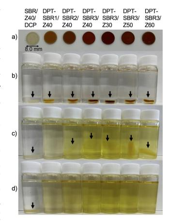
Fig. 8 Photographs documenting the dissolution and swelling behaviour of the cured rubber composites in toluene/dichloroacetic acid (v/v = 95/5): (a) prepared specimens, (b) beginning of the test, (c) after soaking at room temperature for 4 days and (d) after further treatment at 80 °C for 6 h.
