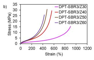
Fig. 11 Engineering stress—strain curves: (a) effect of the amount of bound DPT in the SBRs and (b) effect of loaded ZDMA content.
