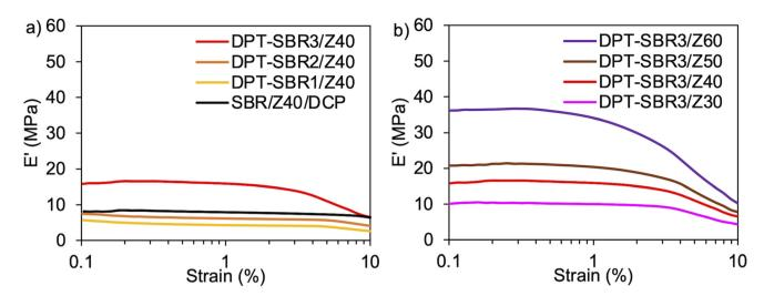
Fig. 10 Strain dependence of E': (a) effect of the amount of bound DPT in the SBR on E' and (b) effect of loaded ZDMA content on E'.
