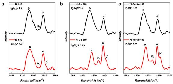
Fig. 4 Raman spectra of the Ni-based electrocatalysts with two different functionalization temperatures of 600 °C and 900 °C for the (a) Ni; (b) Ni-Co; and (c) Ni-Fe-Co samples.
