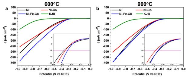
Fig. 11 The LSVs of RDE measurement for the KJB Ni-based electrocatalysts with different compositions of materials and different thermal treatment temperatures of (a) 600 °C and (b) 900 °C in  $N_2$  saturated KOH (1 M) solution. The scan rate of 5 mV s<sup>-1</sup> and a rotating disk speed of 1600 rpm were used for the measurements. The KJB carbon was measured as a control.
