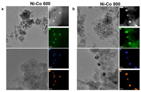
Fig. 2 (a) TEM characterization of the Ni–Co 600 °C and Ni–Co 900 °C samples. For each sample, leftmost top image and bottom image report HRTEM characterization, while the rightmost column reports the STEM EDX mapping. (a) The Ni–Co sample functionalized at 600 °C (Ni–Co 600), and (b) the sample functionalized at 900 °C (Ni–Co 900).
