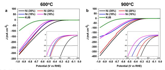
Fig. 9 The LSVs of the RDE measurement of KJB Ni-based electrocatalysts with different wt% of NiPc in their composition, and different thermal treatment temperatures of (a) 600 °C and (b) 900 °C in  $N_2$  saturated KOH (1 M) solution. The scan rate of 5 mV s<sup>-1</sup> and a rotating disk speed of 1600 rpm were used for the measurements. The KJB carbon was measured as a control.
