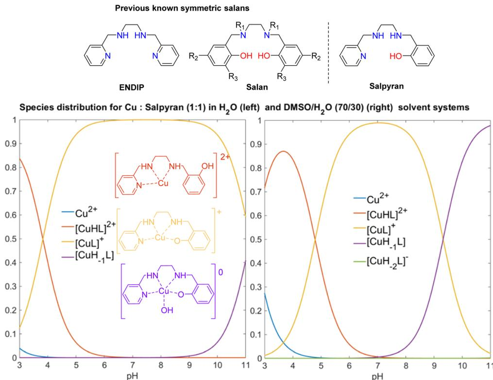
**Fig. 10** A comparison of the known tetradentate ligands and salpyran and species distribution of the Cu:salpyran dynamic system in 1 : 1 ratio at a different solvent system, emphasising the solvent impact on species formation. Adapted from ref. 68 with permission from Copyright 2021 American Chemical Society.
