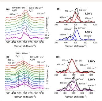
Operando Raman spectra of the Mn(II) (a) and (b) and Mn(IV) (c) and (d) phase in 0.1 M KOH. Fitted spectra (b) and (d) at two selected potentials below and above the oxygen evolution potential. Potentials are vs. the reversible hydrogen electrode (RHE). Figure adapted from ref. 56 under CC BY 4.0 license
