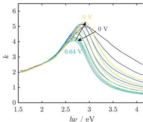
Fig. 5 UV/Vis spectra of thin  $\text{MnO}_x$  films, represented by the imaginary part  $k$  of the complex refractive index, at pH 13 during electrochemical cycling show reversible peak shifts. In this example, the OER onset was observed at  $\approx 0.55\text{ V}$  vs.  $\text{Ag}/\text{AgCl}/3\text{ M KCl}$ . Figure adapted from ref. 32 under CC BY 3.0 license.
