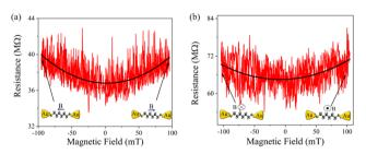
Fig. 3 The observed MR effect of the Au/HDT/Au junction in (a) parallel and (b) perpendicular magnetic field orientation with respect to the current direction
