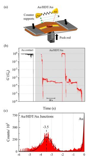
Fig. 1 (a) Scheme of the MCBJ technique and the structure of Au/HDT/ Au. (b) Representative G transient curves obtained for the contact of bare and HDT-modified Au. (c) Histogram of G transient curves for HDT-modified Au showing the most probable conductance peak.
