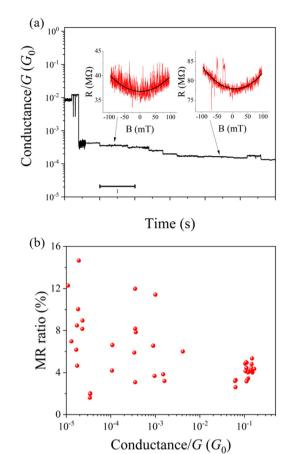
Fig. 2 (a) A G transient curve of Au/HDT/Au and the MR curves with the parabolic fit (inset). (b) The plot of MR ratio as a function of G for Au/HDT/Au
