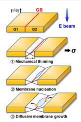
Fig. 8 A sketch of the mechanical thinning mechanism of the formation of a 2D gold membrane using in situ TEM. Reproduced with permission from ref. 97. Copyright © 2020 American Chemical Society
