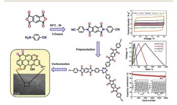
Fig. 6 Schematic of the synthesis of p-TIDN and the electrochemical performance of p-TIDN in a two-electrode system in TEABF<sub>4</sub>/AN. Reproduced from ref. 111 with permission from Elsevier, Copyright 2020
