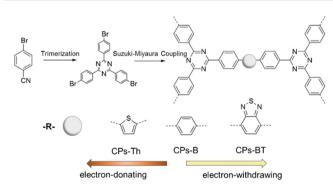
Fig. 4 Synthesis of CTFs by Suzuki cross-coupling. Reproduced from ref. 76 with permission from Elsevier, Copyright 2018.
