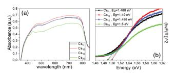
Fig. 9 (a) UV-vis absorption spectra and (b) Tauc plots of the Cs doped, MA-free perovskite films under study
