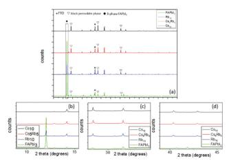
Fig. 1 X-ray diffraction patterns of the perovskite films (a) at full range and (bottom) with a focus at  $10-15^\circ$  (b),  $28-33^\circ$  (c), and  $42-46^\circ$  (d). The " $\nabla$ " denotes the perovskite peaks and "\*" denotes the fluorine-doped tin oxide (FTO) peaks
