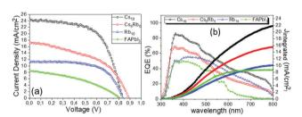
Fig. 3 (a) Current density-voltage curves of the champion C-PSCs, incorporating the MA-free perovskites under study, under illumination of 100 mW cm<sup>-2</sup> simulated sun irradiation (1.5 AM) and (b) EQE of the corresponding solar cells.
