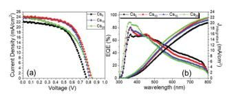
Fig. 10 (a) Current density-voltage curves of the highest performing C-PSCs, incorporating the Cs doped, MA-free perovskites under study, under illumination of 100 mW cm<sup>-2</sup> simulated sun irradiation (1.5 AM) and (b) EQE of the corresponding solar cells
