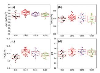
Fig. 11 Statistical graphs illustrating the device performance statistics (>20 devices for each condition) for C-PSCs incorporating the MA-free perovskites under study (a)  $J_{\rm sc}$ , (b)  $V_{\rm oc}$ , (c) FF, and (d) PCE, represented in box-and-whisker plots. Device parameters are obtained from reverse J-V scans.
