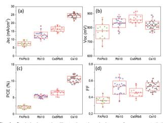
Fig. 4 Statistical graphs illustrating the device performance statistics (20 devices for each condition) for C-PSCs incorporating the MA-free perovskites under study (a)  $J_{\rm sc}$ , (b)  $V_{\rm oc}$ , (c) PCE, and (d) FF, represented in box-and-whisker plots. Device parameters are obtained from reverse J-V
