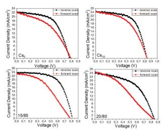
Fig. 12 J-V curves of the highest performing C-PSCs prepared with the Cs doped, MA-free perovskites under study, in forward and reverse
