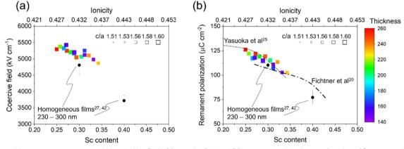
Fig. 4 Composition-structure-property relations in Al<sub>1-x</sub>Sc<sub>x</sub>N: (a) coercive field and (b) remanent polarization as a function of Sc content along with c/a and thickness in library, compared to reported homogeneous films. 20,25,27,42
