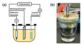
Fig. 1 (a) Schematic diagram of an electrodeposition apparatus: ITO as the working electrode, platinum coil as the counter electrode, and an Ag/AgCl electrode as the reference electrode. (b) A photo of an electrodeposition setup.
