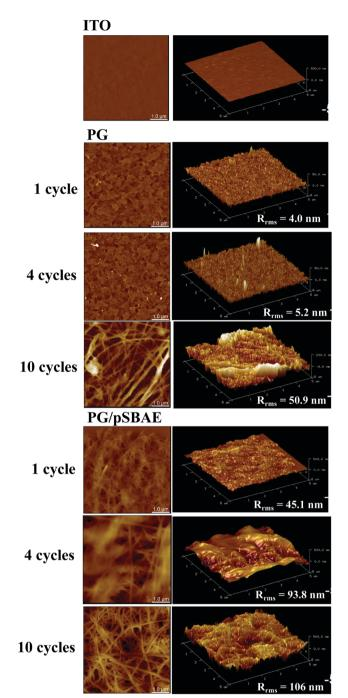
Fig. 4  $\,$  AFM images of surface topography of bare ITO, and ITO electrodeposited with PG and PGSB for 1, 4 and 10 cycles. Scale = 1.0  $\mu m$ .
