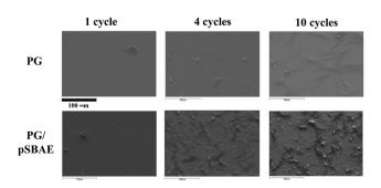
Fig. 3 The SEM images of electrodeposited PG and PG/pSBAE coatings on ITO for 1, 4 and 10 cycles.
