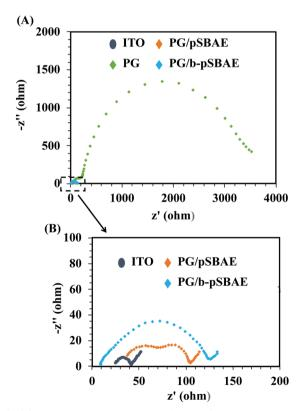
Fig. 6 (A) Impedance Nyquist plots of the EIS obtained at different modified electrodes: ITO, PG (8 mg mL<sup>-1</sup>), PG/pSBAE and PG/b-pSBAE  $(8/30 \text{ mg mL}^{-1})$ . (B) The enlarged figure from the enclosed area in (A). Measurements were performed in PBS containing 10 mM [Fe(CN)<sub>6</sub>]<sup>3-</sup>/<sup>4-</sup> and 0.1 M KCl.
