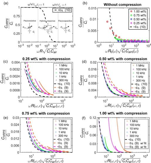
Fig. 4 (a) A master curve based on eqn (10) that can capture all three regimes – piezoresistive, hybrid, and piezocapacitive responses. (b) Frequency-only validation of the master curve (black dashed curve). The colored dashed and dotted curves are based on eqn (9). Note that as the compressive strain increases, the x axis  $\omega R \sqrt{C_i C_{\text{nir}}}$  goes left.
