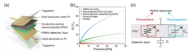
Fig. 1 (a) A schematic showing the layers of the HRPS.<sup>24</sup> (b) The HRPS is much more sensitive than the conventional CPS.<sup>24</sup> (c) A simplified circuit model to represent the hybrid piezoresistive and piezocapacitive responses of the HRPS. (a and b) Reproduced from ref. 24 with the permission of Wiley.
