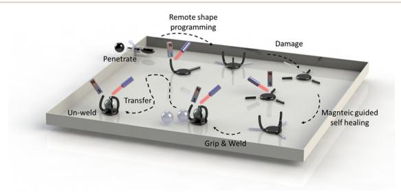
Fig. 1 A magnetic vitrimer-based soft robot can squeeze itself to pass through an extremely confined space, reshape, self-heal, grip, transport and release an object.
