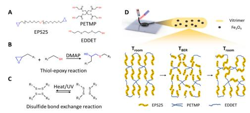
Fig. 2 Preparation and the molecular structure of the magnetic vitrimer used in the current study. (A) Molecular structure of the monomer EPS25, crosslinker PETMP and chain extender EDDET. (B) Crosslinking mechanism of the thiol-epoxy reaction with DMAP (4-dimethylaaminopyridine) as the catalyst. (C) Mechanism of the disulfide bond exchange reaction. (D) Reconfiguration mechanism of the magnetic vitrimer.
