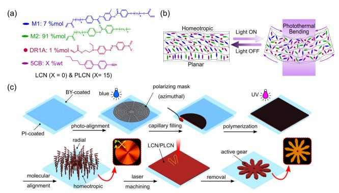
Fig. 3 (a) Molecular structure of constituent molecules in LCN and PLCN; (b) mechanism of photothermal bending deformation in LC-based crosslinked networks; (c) fabrication schematic view of the LCN gears fabrication with pre-determined molecular alignment. Molecules are aligned radially adjacent to the side of the cell that is exposed to polarized light. Molecules are aligned homeotropically on the other side of the film.
