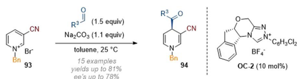
Scheme 27 Enantioselective dearomative C-4 acylation of 3-cyano pyridiniums using NHC catalysis. 33
