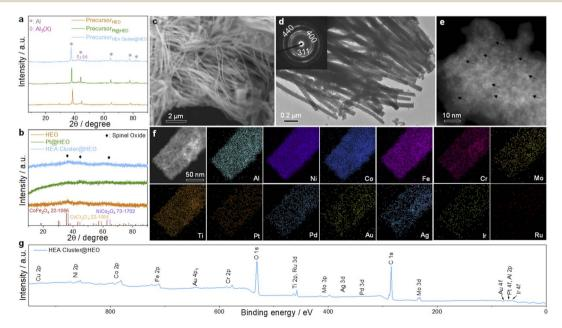
Fig. 1 Characterization of the HEA cluster@HEO. (a) XRD patterns of the precursor alloys and (b) the dealloyed samples. The PDF standard cards of  $CoFe_2O_4$ ,  $CoCr_2O_4$ , and  $NiCo_2O_4$  are included for comparison. (c) SEM, (d) TEM, and (e) HAADF-STEM images and (f) STEM-EDS mapping of the HEA cluster@HEO. Cu was not included because of the interference from the Cu grid. (g) XPS spectrum of the HEA cluster@HEO sample.
