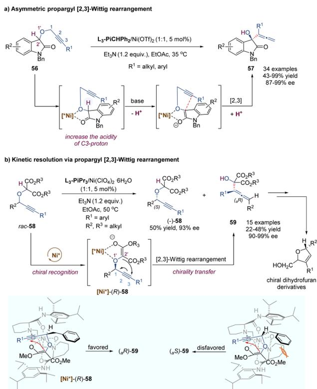
Scheme 19 Nickel-catalysed asymmetric [2,3]-Wittig rearrangement of propargylic ethers.
