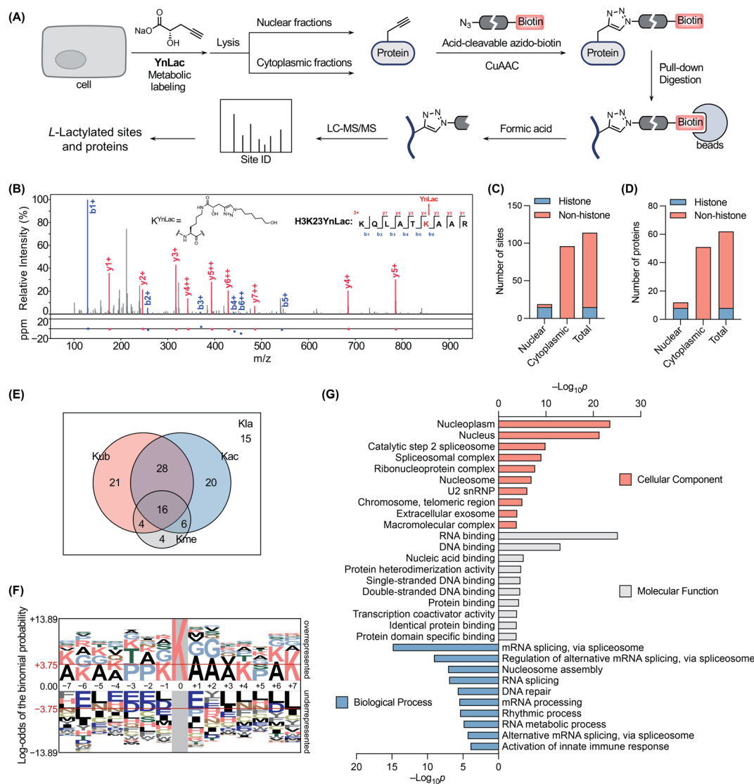
Fig. 3 Chemical proteomic profiling of protein lactylation with YnLac. (A) Workflow for the chemical proteomic profiling of lactylation sites using YnLac. HEK293T cells were metabolically labelled with YnLac and the nuclear and cytoplasmic fractions were separated for click conjugation with acid-cleavable azido-biotin and affinity pull-down. After on-bead digestion, the peptides were eluted with acid and analyzed by MS. (B) A representative MS/MS spectrum shows the identification of YnLac modification on the K23 residue of histone H3. (C) Summary of identified lactylation sites in the nuclear and cytoplasmic fractions. (D) Summary of identified lactylated proteins in the nuclear and cytoplasmic fractions. (E) The Venn diagram shows the overlap of identified lactylation sites (Kla) with three abundant types of lysine PTMs, i.e. , acetylation (Kac), ubiquitination (Kub), and methylation (Kme). (F) Sequence motif analysis shows the preference of amino acid residues around the identified lactylation sites. The red horizontal lines denote thresholds of p < 0.05 . (G) GO term enrichment analysis of identified lactylated proteins.
