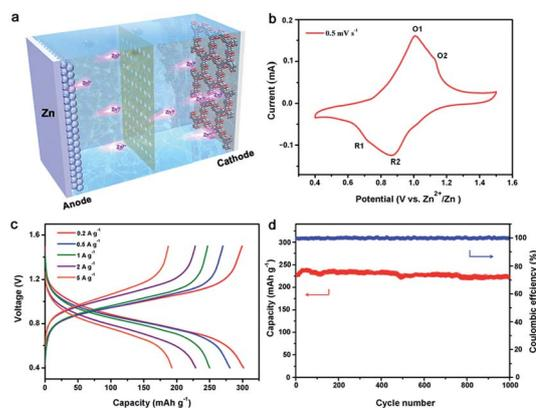
**Fig. 3** (a) Illustration of the aqueous Zn/Tp-PTO-COF battery; (b) CV curve at a scan rate of  $0.5 \text{ mV s}^{-1}$ ; (c) galvanostatic charge–discharge curves of the aqueous Zn/Tp-PTO-COF battery at various current densities; (d) cycle stability at a current density of  $2 \text{ A g}^{-1}$ .
