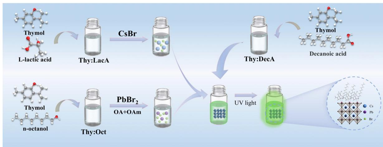
Fig. 1 Schematic illustration of synthetic procedure for NADES-CsPbBr<sub>3</sub> PNCs.
