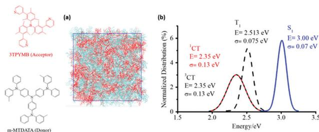
**Fig. 4** (a) Illustration of the simulated morphologies of the m-MTDATA:3TPYMB blend. (b) Distributions of the calculated energies of the lowest CT and LE singlet and triplet states.
