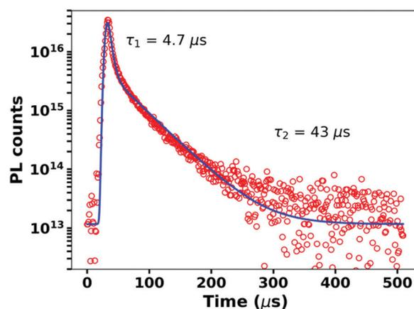
Fig. 2 Time-resolved PL decay of the m-MTDATA/3TPYMB blend (red circles) shows prompt and delayed emission with time constants of 4.7  $\mu$ s and 43  $\mu$ s. A bi-exponential function convolved with experimental IRF is fit to the data and shown in blue.
