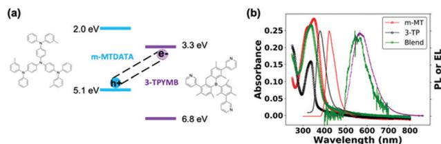
Fig. 1 (a) State energies<sup>31</sup> and molecular structures of m-MTDATA and 3TPYMB. (b) Absorption (–o–) and PL spectra (–) of neat donor (red), acceptor (black) and blend films/devices (green) overlaid with EL spectrum (purple) of the blend device. The PL spectrum of the blend was measured from the solar cell device stack.
