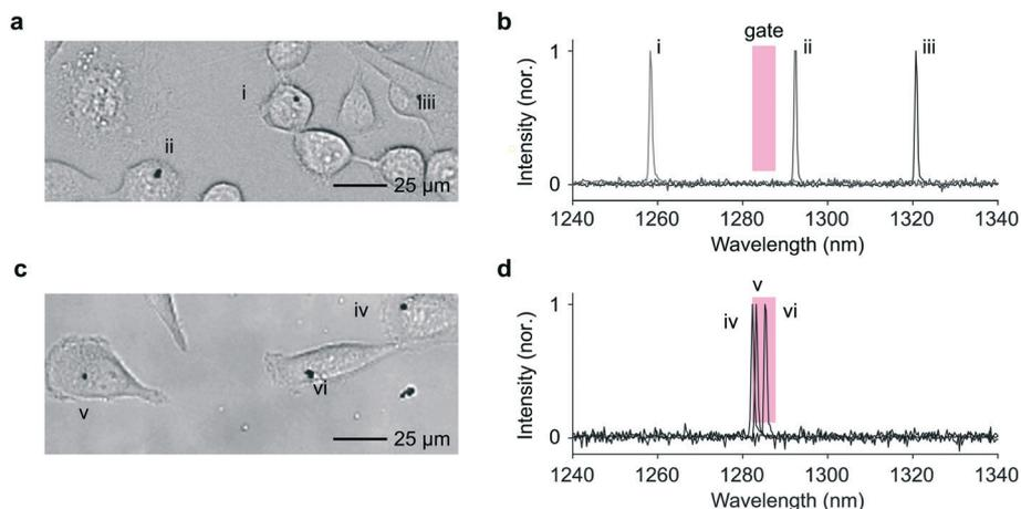
**Fig. 6** Band-pass sorting. a, A bright-field image of replated cells collected from the (-) outlet. b, The LP lasing emissions from the LPs labelled i, ii and iii. c and d, Image and emission spectra of cells collected from the (+) outlet, showing three LPs (iv–vi).
