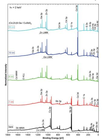
Fig. 1 HAXPES survey spectra recorded with 2 keV of the bare CuSbS<sub>2</sub> absorber (bottommost spectrum) and of the (Cd,Zn)S:Ga/CuSbS2 samples with buffer thicknesses varying from 1 nm (spectrum second from the bottom) to 50 nm (topmost spectrum). Vertical offsets were added for clarity.
