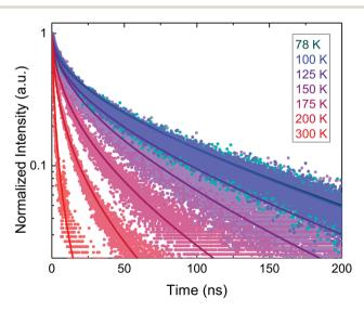
Fig. 4 TRPL spectra measured on a Ba<sub>3</sub>Zr<sub>2</sub>S<sub>7</sub> crystal for temperature between 78 and 300 K, measured with pump wavelength 705 nm and pump fluence of 3.85 mJ cm<sup>-2</sup> (1.37  $\times$  $10^{16}$  ph cm $^{-2}$ ) per pulse. The TRPL data (points) and best-fit models (lines) are normalized to accentuate the rise in decay rate with increasing temperature.
