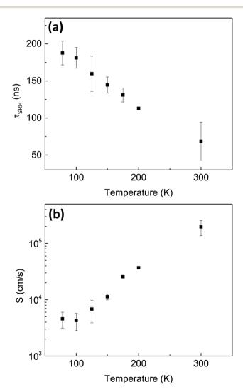
Fig. 5 Temperature-dependence of (a)  $\tau_{SRH}$ , and (b) S, for Ba<sub>3</sub>Zr<sub>2</sub>S<sub>7</sub> determined from the data and models shown in Fig. 4.
