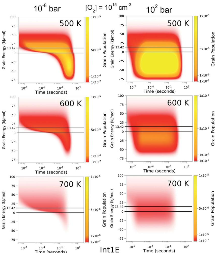
Fig. 12 The time-dependent energy grain populations of Int1E at  $10^{-8}$  bar and  $10^2$  bar between 500 K and 700 K. The horizontal lines show where the relative energies of the reactants and ts1EP1E are.
