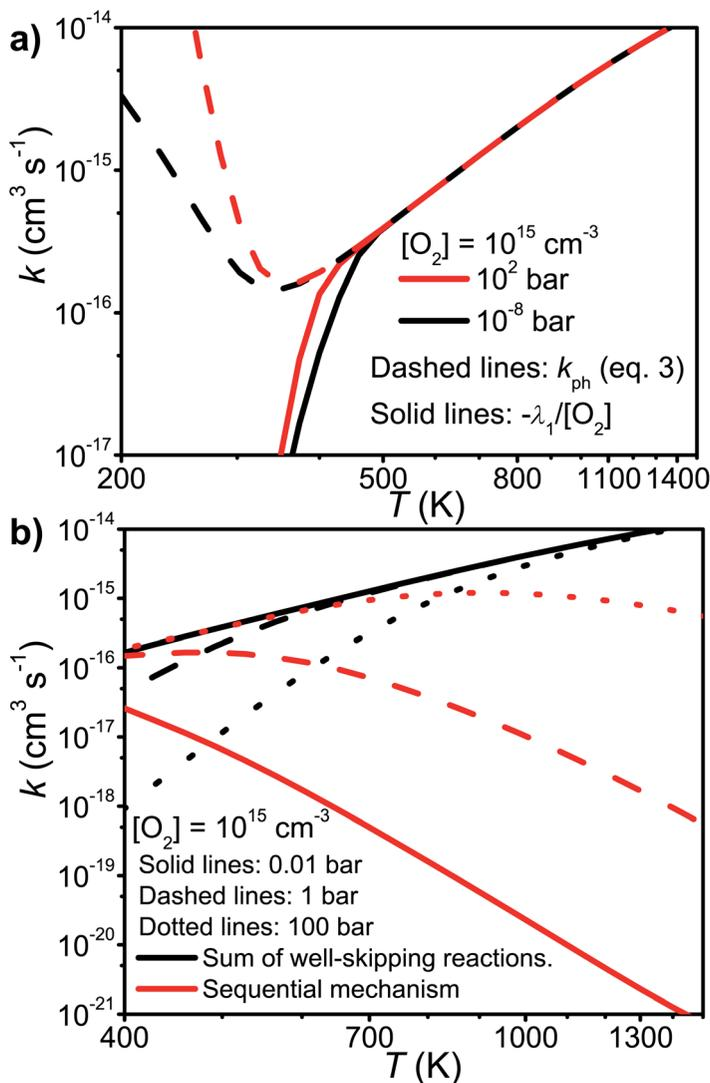
Fig. 9 (a) A comparison of the phenomenological rate coefficient given by eqn (3) and  $-\lambda_1/[\text{O}_2]$ . (b) The sum of the well-skipping rate coefficients in eqn (3) and the sequential mechanism plotted as a function of temperature and pressure (see text for details).
