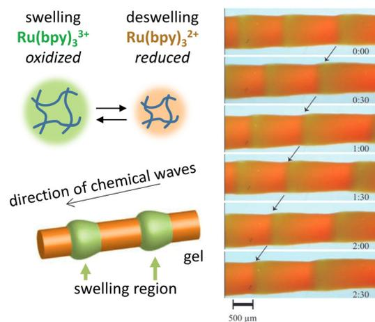
Fig. 4 Functional oscillating systems based on the Belousov–Zhabotinsky (BZ) reaction. By incorporating the BZ reaction into a hydrogel, the hydrophilicity change resulting from  $\text{Ru}^{2+}$ – $\text{Ru}^{3+}$  switching can be exploited to cause periodic swelling and deswelling, giving rise to peristaltic motion. Reproduced from ref. 77 with permission from the Wiley-VCH publishing group, Copyright 2008.
