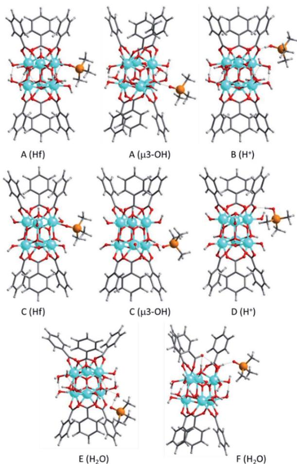
Fig. 5 Optimized geometries of TMPO interacting with Hf Lewis sites,  $\mu_3$ -OH Brønsted acid sites, or additional  $\text{H}_2\text{O}$  molecules, and of protonated  $\text{TMPOH}^+$  in Hf-MOF-808 models. The labels A to F identify the MOF-808 model used, as described in Fig. S1,† and the type of interaction between TMPO and MOF-808 is given in parenthesis. C and O atoms are depicted as gray and red sticks, Hf, P and H as cyan, yellow and white balls.
