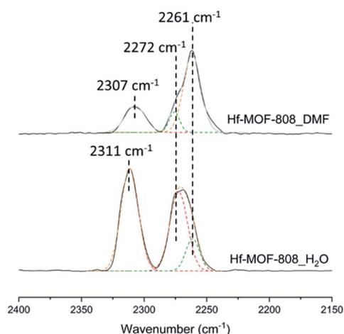
**Fig. 3** FTIR spectra of 2 mbar CD<sub>3</sub>CN adsorbed at 25 °C on Hf-MOF-808-H<sub>2</sub>O (down) and Hf-MOF-808-DMF (top). The IR bands at 2311 and 2307 cm<sup>-1</sup> are associated with CD<sub>3</sub>CN coordinated to Hf sites, and the IR bands at 2272 cm<sup>-1</sup> to OH groups in the Hf cluster. The band at 2261 cm<sup>-1</sup> is associated with physisorbed CD<sub>3</sub>CN molecules.
