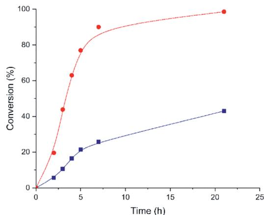
Fig. 8 Kinetic profiles for styrene oxide conversion employing Hf-MOF-808\_H<sub>2</sub>O (red circles) and Hf-MOF-808\_DMF (blue squares) as catalysts.
