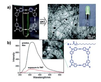
Fig. 12 (a) Fabrication of macrocycle-based nanofibril upon gelation. (b) The fluorescence quenching of the nanofibril film after exposure to TNT. Reproduced with permission: (a) from ref. 68, Copyright 2006, The American Chemical Society; (b) from ref. 69, Copyright 2007, The American Chemical Society.
