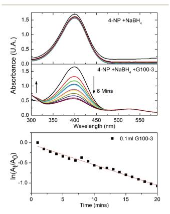
Fig. 6 UV-Vis absorbance spectral kinetics of 4NP + NaBH<sub>4</sub> (top panel) and 4NP + NaBH<sub>4</sub> + G100-3 (center). The variation of  $\ln(A_t/A_0)$  versus time, where  $A_t$  is the absorbance at 400 nm at a given time and  $A_0$  is the absorbance value t time t=0 min.
