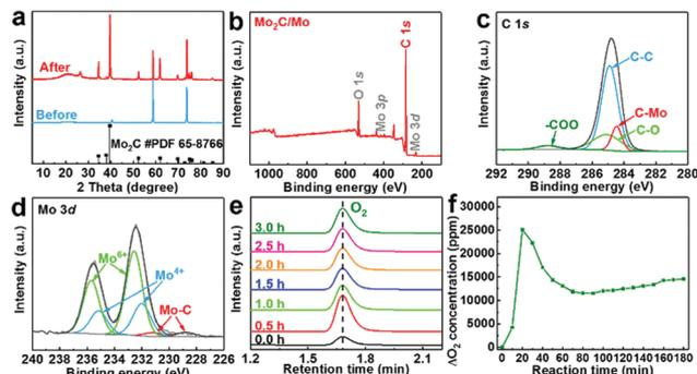
Fig. 3 (a) XRD patterns of  $\text{Mo}_2\text{C}/\text{Mo}-60$  and Mo film. (b) XPS survey spectrum of the  $\text{Mo}_2\text{C}/\text{Mo}-60$ . High-resolution C 1s (c) and Mo 3d (d) XPS spectra for  $\text{Mo}_2\text{C}/\text{Mo}-60$ . (e) Gas chromatogram of oxygen flowing out from the experimental system at different times. (f) Variation of oxygen concentration during electrolysis at 3.1 V.
