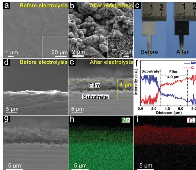
Fig. 2 Typical SEM images for the surfaces of the Mo plate (a) and obtained  $\text{Mo}_2\text{C}/\text{Mo}-60$  (b). (c) Digital photos of Mo plates before and after electrolysis. Cross-sectional SEM images of Mo (d) and  $\text{Mo}_2\text{C}/\text{Mo}-60$  (e). Corresponding EDS results of linear sweep analysis (f) and elemental distribution mappings (g–i) for  $\text{Mo}_2\text{C}/\text{Mo}-60$ .
