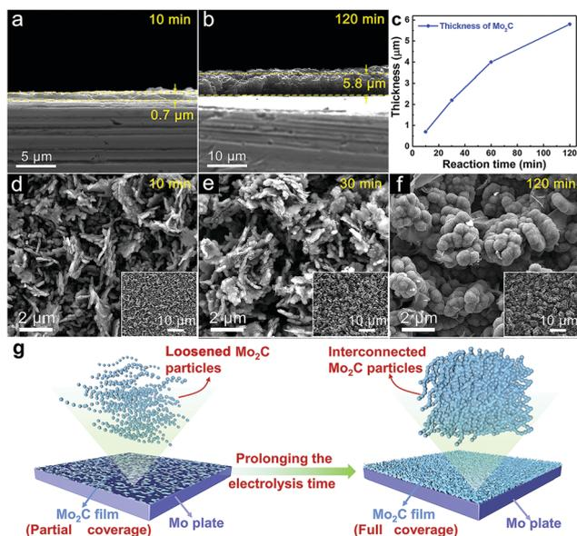
**Fig. 4** Cross-sectional SEM images of  $\text{Mo}_2\text{C}/\text{Mo}$ -10 (a) and  $\text{Mo}_2\text{C}/\text{Mo}$ -120 (b). (c) Thickness change of the  $\text{Mo}_2\text{C}$  layer vs. electrolysis time. SEM images of  $\text{Mo}_2\text{C}/\text{Mo}$ -10 (d),  $\text{Mo}_2\text{C}/\text{Mo}$ -30 (e) and  $\text{Mo}_2\text{C}/\text{Mo}$ -120 (f). (g) Illustration of the changes of thickness and morphology of the  $\text{Mo}_2\text{C}$  film by prolonging the electrolysis time.
