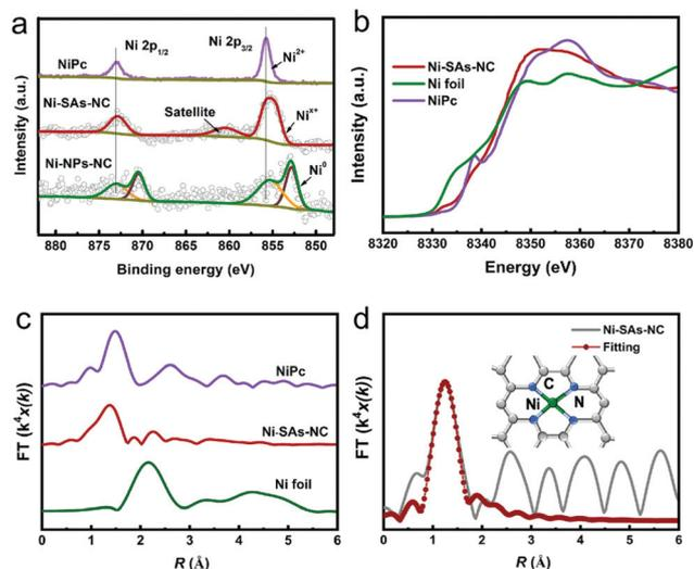
**Fig. 2** (a) Ni 2p XPS spectra of NiPc, Ni-SAs-NC and Ni-NPs-NC. (b) Ni K-edge XANES spectra of Ni-SAs-NC, NiPc and Ni foil. (c) Fourier-transformed EXAFS spectra of Ni-SAs-NC, NiPc, and Ni foil. (d) Fourier-transformed EXAFS fitting results of Ni-SAs-NC (inset shows the proposed structural model of Ni-SAs-NC).
