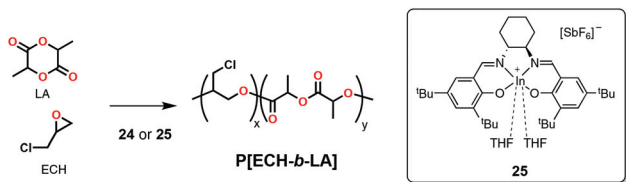
Scheme 23 Cationic indium complex active in the block copolymerization of epichlorohydrin and lactide through the simultaneous addition of monomers.
