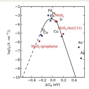
Fig. 8 Volcano plot of various elements with respect to  $\Delta G_{H^*}$ . Reproduce from ref. 129.
