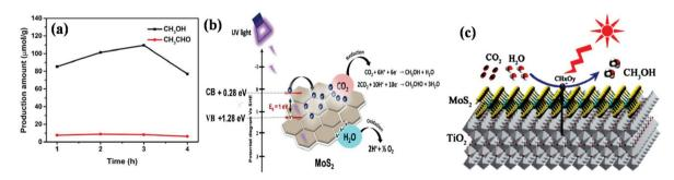
Fig. 14 (a) Rate of CO<sub>2</sub> reduction by MoS<sub>2</sub> sheets in 0.5 M NaHCO<sub>3</sub> and (b) schematic representation of the mechanistic pathway for photocatalytic CO<sub>2</sub> reduction over MoS<sub>2</sub> sheets. Reproduced with permission.<sup>173</sup> (c) Schematic illustration of the photoreduction of CO<sub>2</sub> to CH<sub>3</sub>OH in the MoS<sub>2</sub>/ TiO<sub>2</sub> heterostructure. Reproduced with permission. 170
