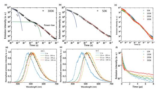
Fig. 2 Emission decay profiles in a log-log plot of the m-MTDATA/PPT film at 300 K (a), 50 K (b), and various temperatures (c). Solid lines show fitting of  $\tau_{\rm P}$ ,  $\tau_{\rm d}$ , and power-law decay. Time-dependent emission spectra at 300 K (d) and 50 K (e). Emission decay profiles in a semi-log plot (f).
