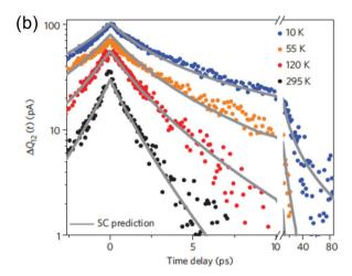
Fig. 9 (a) Schematic illustration of cooling via acoustic phonons without (left) and with (right) disorder, where the presence of disorder speeds up the emission of acoustic phonons, also known as "supercollision cooling".85 (b) Experimental measurements of cooling dynamics using time-resolved photocurrent microscopy, together with calculations using disorder-assisted acoustic phonon cooling. Panels (a) and (b) are adapted with permission from ref. 33 (Copyright 2013 Springer Nature).
