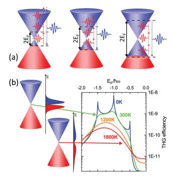
Fig. 13 (a) THG in graphene is enhanced at specific values of  $E_{\rm F}$  corresponding to one-, two- and three-photon transitions within the Dirac cone. (b) The increase of  $T_{\rm e}$  affects the nonlinear conversion efficiency by broadening the electron distribution. The graph shows the THG efficiency, defined as  $I_{3\omega}/I_{\omega}$ , for  $\hbar\omega$  = 500 meV and a peak power density of  $\sim$ 230 MW cm<sup>-2</sup>.
