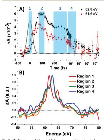
Fig. 3 (A) Time traces (data points). Error bars are  $\pm$  the standard error. Data traces are integrated  $\pm 0.2$  eV from the listed value. Four integration regions (light blue) are defined. The 48 fs instrument response function is plotted in grey. (B) Normalized and smoothed (5-point [1.0 eV] Savitzky–Golay) time-averaged regions.
