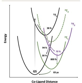
Fig. 6 Schematic representing potential energy surfaces in the proposed model.
