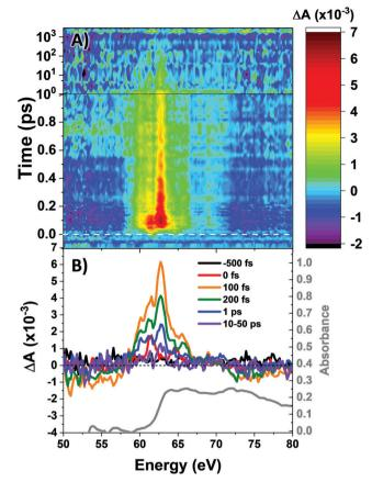
Fig. 2 (A) Contour plot of time-resolved M-edge XANES spectra. Time zero is indicated in the dashed white line. (B) Selected spectral slices with the ground state Co<sub>4</sub>O<sub>4</sub> spectrum in grey for comparison. The data are binned to 0.2 eV intervals
