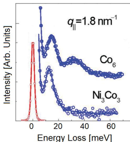
Fig. 7 HREELS spectra with magnon excitations for  $\text{Co}_6$  and  $\text{Ni}_3\text{Co}_3$  films grown on  $\text{Cu}(100)$ , with correction to account the Bose occupation number. Adapted from ref. 95.
