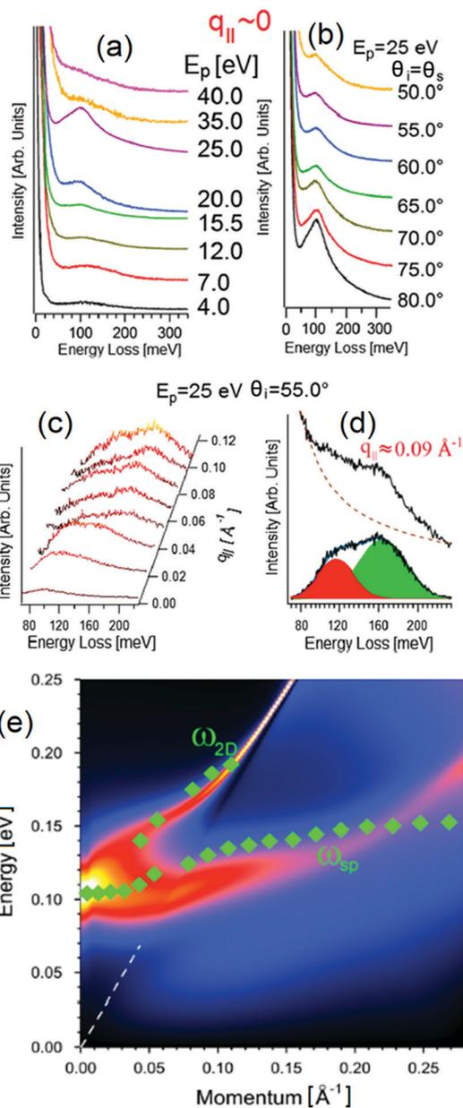
Fig. 6 Dependence on (a) primary electron beam energy (taken in specular direction with the incidence angle of  $55^\circ$ ) and (b) scattering geometry of the HREELS spectrum in Bi<sub>2</sub>Se<sub>3</sub>. (c) Momentum-resolved HREELS spectra; (d) fit procedure showing the presence of two well-distinct plasmonic excitations; (e) dispersion relation of the Dirac and surface plasmon. Adapted from ref. 73.
