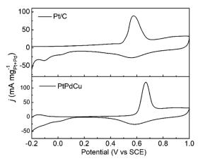
Fig. 7 CO stripping voltammograms of PtPdCu and Pt/C catalysts in 0.5 mol  $L^{-1}$  H<sub>2</sub>SO<sub>4</sub> at 50 mV s<sup>-1</sup>.
