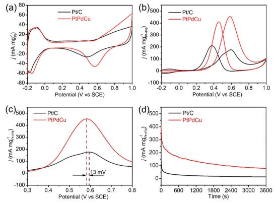
Fig. 6 (a and b) CVs of Pt/C and PtPdCu cubic nanoframes in 0.5 mol  $L^{-1}$  N<sub>2</sub>-saturated H<sub>2</sub>SO<sub>4</sub> solution and in 0.5 mol  $L^{-1}$  H<sub>2</sub>SO<sub>4</sub> mixed with 0.5 mol  $L^{-1}$  methanol; (c) enlarged view of the peaks at 0.6 V in (b); (d) chronoamperograms of Pt/C and PtPdCu cubic nanoframes in 0.5 mol  $L^{-1}$  H<sub>2</sub>SO<sub>4</sub> mixed with 0.5 mol  $L^{-1}$  methanol.
