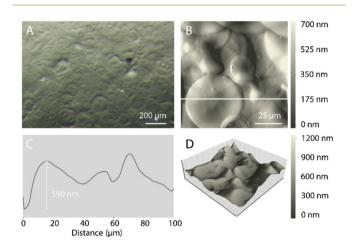
Fig. 2 A typical area of glass support covered with a 1 wt% HEC solution observed with an (A) optical and (B) atomic force microscope. (C) Line scan corresponding to the line in B, showing the height profile of the HEC on the surface of the glass substrate. (D) 3D view of the area in В.
