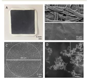
Fig. 3 (A) Optical image of a typical piece of SERS-paper. (B) (top) SEM images of filter paper sprayed with 16 mL of a concentrated aggregated HRSC in 0.6 wt% HEC solution and (bottom) 100 mL of the optimised SERS-paper 1 wt% HEC aggregated CRGC solution. (C) SEM image showing the distribution of nanoparticle aggregates within a 60 µm diameter laser spot in the SERS-paper substrate. (D) SEM image showing the aggregates in the HEC matrix of the SERS-paper at high magnification.
