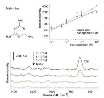
Fig. 8 SERS intensity of different concentrations of aqueous melamine solutions with albumin applied from the paper (orange) or the nanoparticle (purple) side of the SERS-paper. Data points are an average over 5 measurements and error bars represent the SD. Lines are obtained using a best fits log function (top). The SERS spectra of several solutions of melamine contaminated with albumin applied to the paper side of the substrate show the detection limit of  $5 \times 10^{-5}$  M (bottom).
