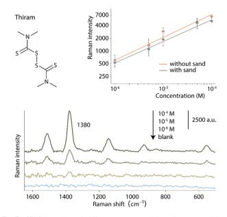
Fig. 7 SERS intensity of different concentrations of aqueous thiram solutions with (grey) and without (orange) sand contamination, both applied from the paper side of the SERS-paper. Data points are an average over 5 measurements and error bars represent ±1 SD. Lines are obtained using a best fit log function (top). The SERS spectra of several solutions of thiram contaminated with sand applied to the paper side of the substrate show the detection limit of 10<sup>-6</sup> M (bottom).
