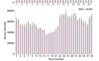
Fig. 5 SERS intensity of the  $268~\rm cm^{-1}$  band in each of the pieces cut from prepared films A (top) and B (bottom). Each data point represents the average value from five SERS spectra and error bars show the RSD. The RSD of the average values were 19.1% for film A and 20.0% for film B.
