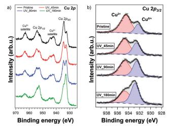
Fig. 5 (a) XPS spectra of the Cu 2p core level region of a pristine (PEA)<sub>2-</sub> CuCl<sub>4</sub> film and after exposing it to UV light for various durations. The film was UV-converted in situ; XPS spectra were recorded after 45, 90 and 180 minutes. (b) Fits of the high-resolution Cu 2p<sub>3/2</sub> peaks with Cu<sup>2+</sup> (red curve) and Cu<sup>0/+</sup> (blue curve) signals for the different data depicted in (a).
