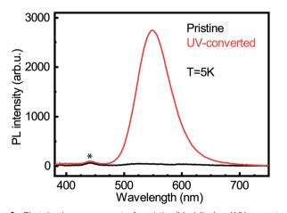
Fig. 6 Photoluminescence spectra for pristine (black line) and UV-converted (red line) (PEA)2CuCl4 films acquired at 5 K. The peak that is marked with an asterisk is a measurement artifact due to stray background light.
