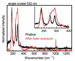
Fig. 2 Raman spectra of a pristine (PEA)<sub>2</sub>CuCl<sub>4</sub> single crystal (black lines) and of the same crystal after 532 nm laser exposure (red lines). The inset displays a magnification of the low-energy part of the spectra
