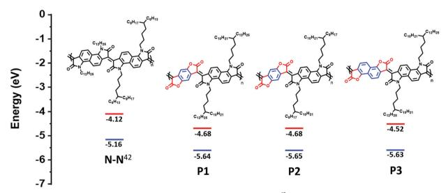
Fig. 1 Chemical structures and calculated HOMO/LUMO of previous studied polymer (N-N)<sup>42</sup> and new polymers, illustrating the effect of introducing bis-lactone units. HOMO is measured by photoelectron spectroscopy in air (PESA). LUMO is calculated from  $E_{opt,qap}$  and IP.
