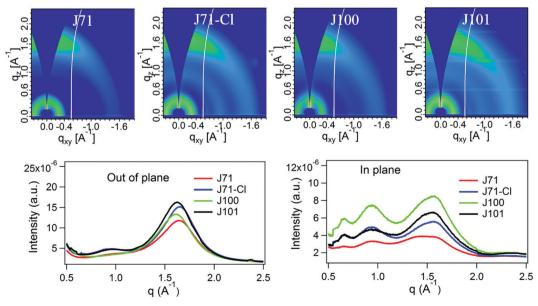
Fig. 2 2D GIWAXS patterns, out-of-plane and in-plane scattering profiles of the four polymers.
