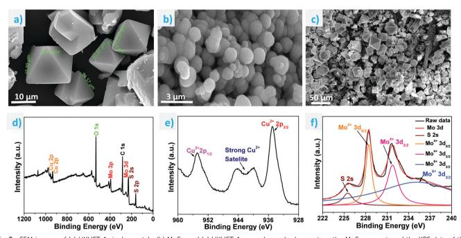
Fig. 2 SEM images of (a) HKUST-1 single crystals, (b) MoS<sub>2</sub>, and (c) HKUST-1 ground sample dropcast on the MoS<sub>2</sub> support, and the XPS data of the  $HKUST-1-MoS_2$  sample; (d) full XPS spectrum; (e) Cu 2p XPS spectrum; and (f) Mo 3d, S 2s XPS spectrum.
