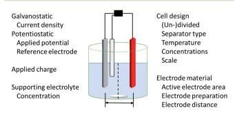
Fig. 3 Crucial parameters for reproducibility in electro-organic synthesis (batch-type).
