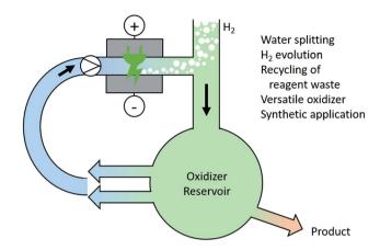
Fig. 6 Anodic generation of high-performance oxidizers during water splitting and their versatile use for synthetic applications.
