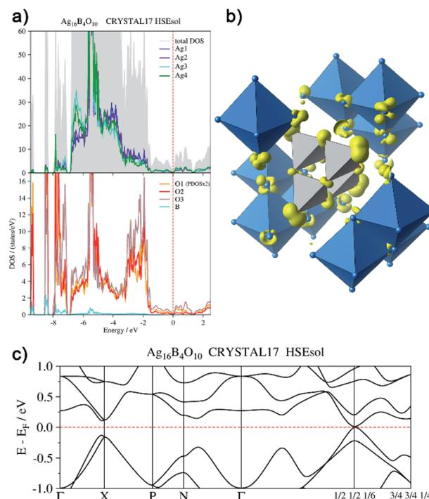
Fig. 7 (a) Total and atom-projected density of states, (b) isosurface ( $0.04 \text{ e}^- \text{ \AA}^{-3}$ ) of the electron density generated by the disperse bands below the Fermi level ( $E_F = -1.44 \text{ eV}$  to  $E_F$ ), (c) bands at  $E_F$ .
