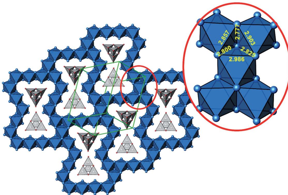
Fig. 4 Cut-out of the crystal structure of  $\text{Ag}_{16}\text{B}_4\text{O}_{10}$ , view along [121]. Magnification (red circle) highlights a block consisting of five edge sharing octahedra with Ag–Ag distances labeled. Same color code as in Fig. 3.
