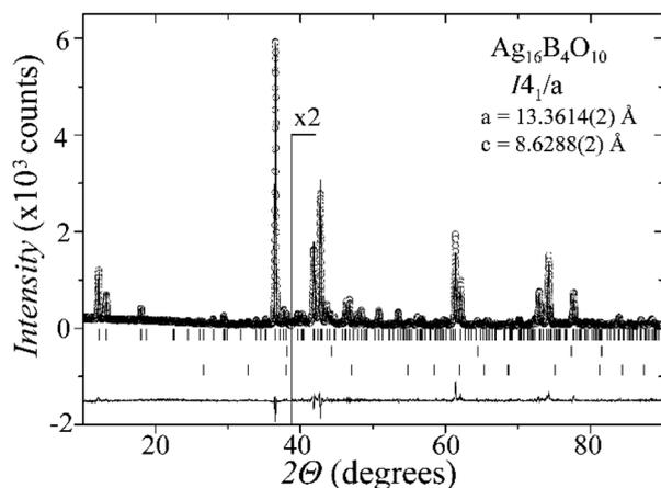
Fig. 1 PXR D pattern of the  $\text{Ag}_{16}\text{B}_4\text{O}_{10}$  sample, showing the observed (circles), Rietveld fit (black line) and difference curve (gray line). The upper, middle and bottom bars mark the reflections for  $\text{Ag}_{16}\text{B}_4\text{O}_{10}$ , Ag and  $\text{Ag}_2\text{O}$ , respectively. The intensity is doubled in the inset for clarity.
