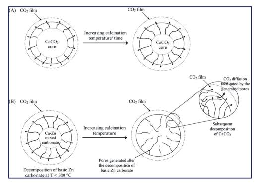
Scheme 3 Proposed models for CaCO<sub>3</sub> decomposition to CaO (A) and mixed precipitate of Ca-Zn (B). Reproduced from ref. 150.
