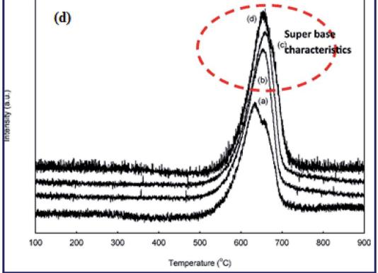
Fig. 17 TEM images and particle size distributions of the surfactant assistant CaO nanocatalysts: after 40 min (a), after 80 min (b), and after 120 min (c).  $CO_2$  desorption performance commercial of CaO (a), and nano CaO catalysts: after 40 min (b), after 80 min (c), and after 120 min (d). Reproduced from ref. 202.
