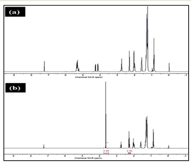
Fig. 23 <sup>1</sup>H NMR spectrum of (a) WCO and (b) Biodiesel. Reproduced from ref. 274.
