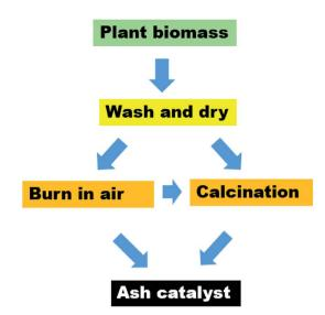
Fig. 19 Flowchart for the synthesis of ash catalyst derived from plant biomass.
