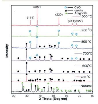
Fig. 18 XRD spectra of normal and calcined (400–1000  $^{\circ}\text{C})$  snail shells. Reproduced from ref. 228.
