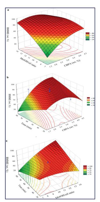
Fig. 22 3-D plots of biodiesel yield. (a) Impact of M/O molar ratio and catalyst loading, (b) reaction time and catalyst loading, and (c) M/O molar ratio and reaction time on the biodiesel yield. Reproduced from ref. 272.
