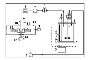
Fig. 7 RPB experimental apparatus utilized for the heterogeneously catalyzed transesterification reaction. Components: (1) CSTR reactor; (2) stirrer; (3) thermocouples; (4) sample port; (5) thermostat; (6) control valve; (7) pumps; (8) flow-meter; (9) RPB reactor; (10) stationary liquid distributor; (11) packed-bed rotator; (12) K/g-Al<sub>2</sub>O<sub>3</sub> catalyst; (13) housing case; (14) rotor shaft; (15) motor. Reproduced from ref. 111
