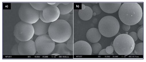
Fig. 32 FESEM images of (a) C and (b) C-SO<sub>3</sub>H. Reproduced from ref. 378.
