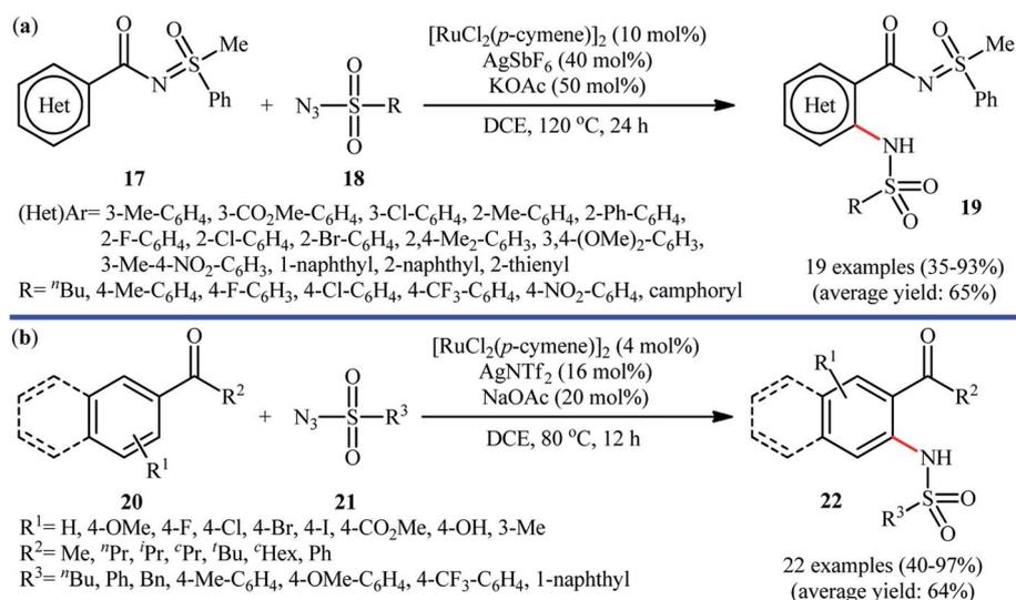
Scheme 6 (a) Sulfoximine directed Ru-catalyzed C–H sulfonamidation of arenes **17** with sulfonyl azides **18**; (b) Ru-catalyzed synthesis of 2-sulfonamidated aromatic ketones **22** from ketones **20** and sulfonyl azides **21**.
