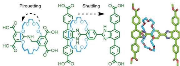
Fig. 43 Schurko and Loeb's [2]rotaxane ligands that form MORFs in which the macrocycle components are able to undergo pirouetting (left) and shuttling (middle; SCXRD structure of methyl ester on right) motion in the solid state.
